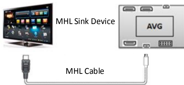
Figure 2.4. Connecting with MHL Sink Device in Stand-alone Mode
