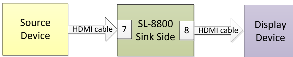
Figure 2.1. Connection Setup for Source Device Testing
